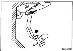
Adjust pedal free play with master cylinder push rod. Then tighten lock nut.
